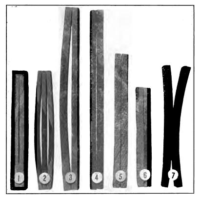
Fig. 65.—Resawed sections cut from casehardened red gum boards steamed for different lengths of time after being kiln dried. (1), No final steaming; (2) and (3), 18 minutes final steaming; (4), (5), and (6), 36 minutes final steaming; (7), 3 hours final steaming.
